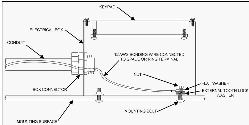
Figure 8 Keypad 314 Rubber/Metal Wire Bonding Example 1
