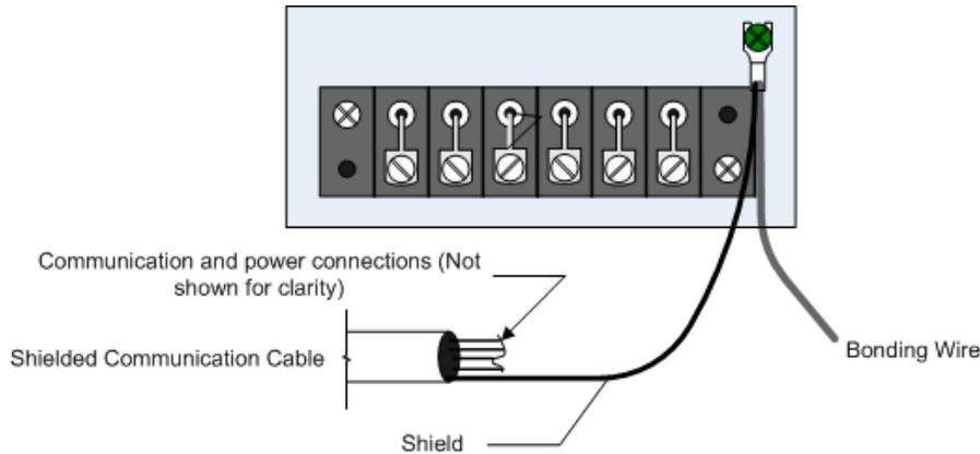
Figure 4 Bonding the Model RS 485 CIM.
