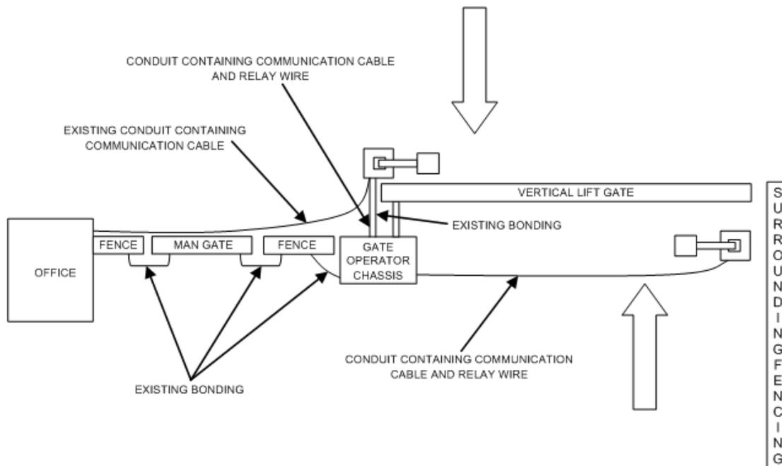
Figure 1 Illustration of a typical gate area.
