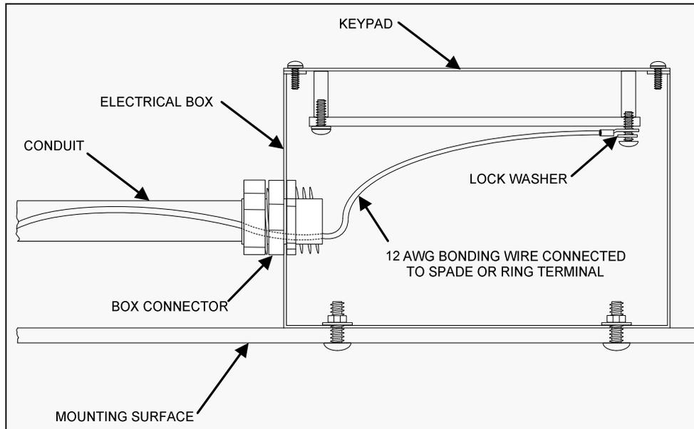
Figure 9 Keypad 314 Rubber/Metal Bonding Example 2
