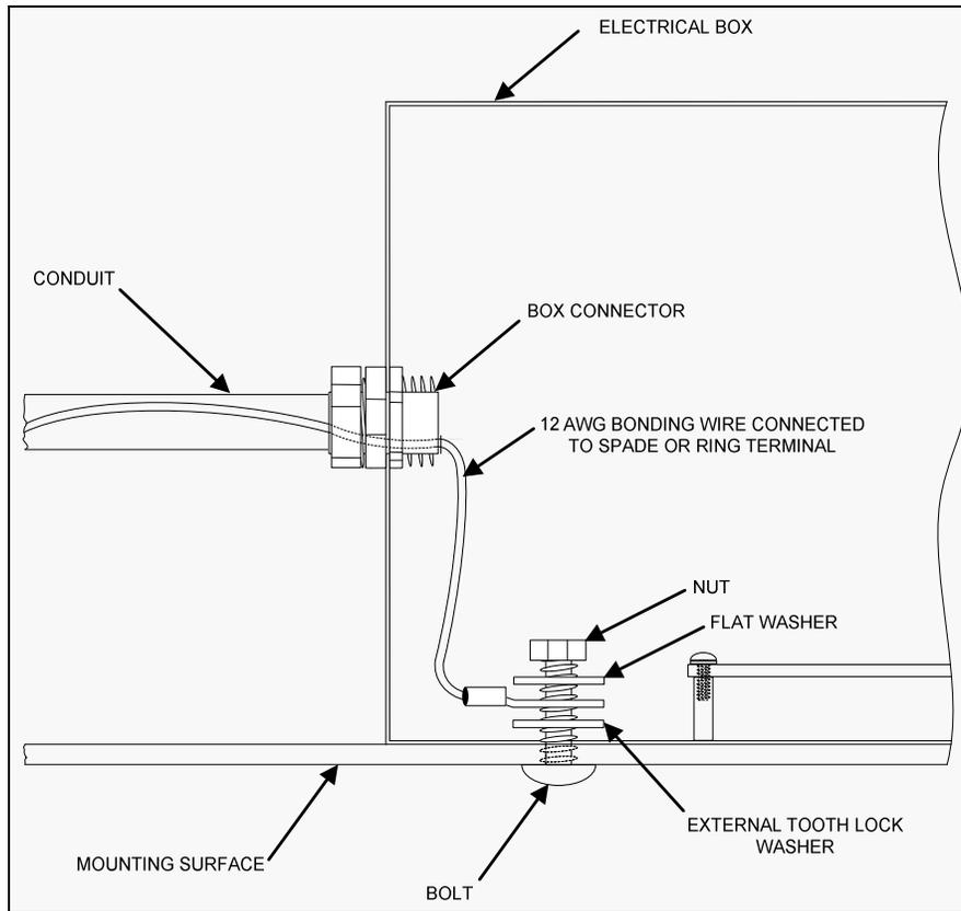
Figure 11 Peripheral Devices (DSB, ECB, CRI) Wire Bonding Example
