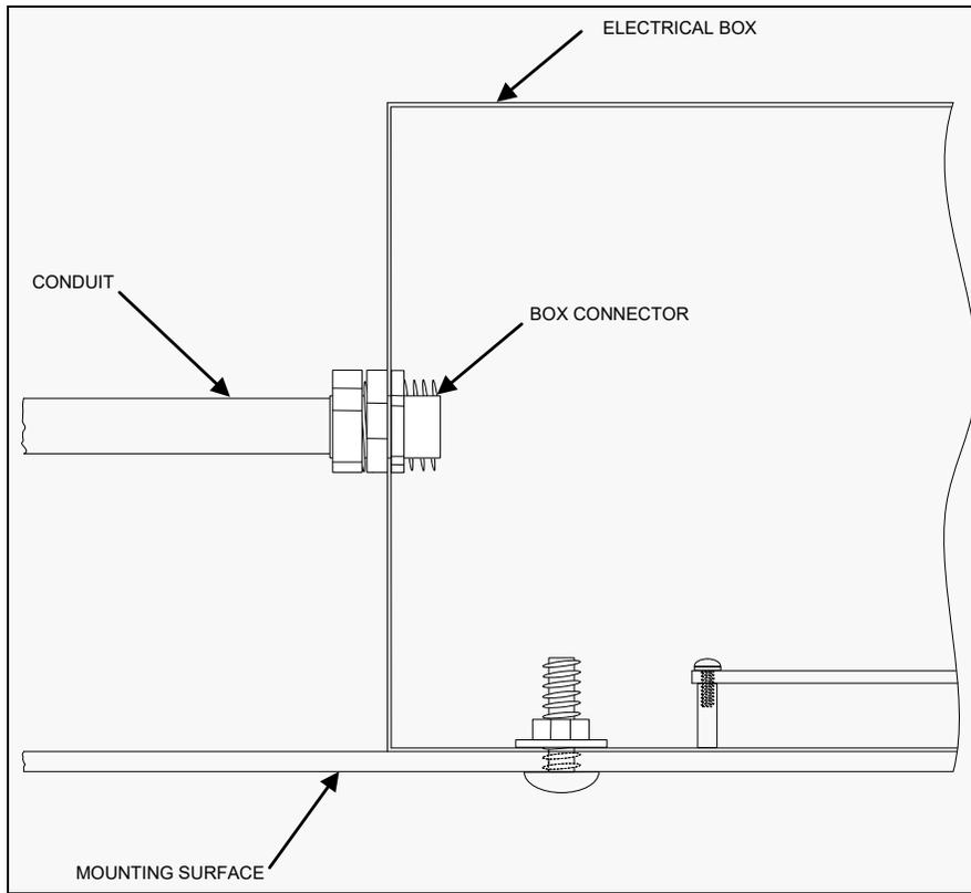
Figure 10 Peripheral Devices (DSB, ECB, CRI) Surface Bonding Example
