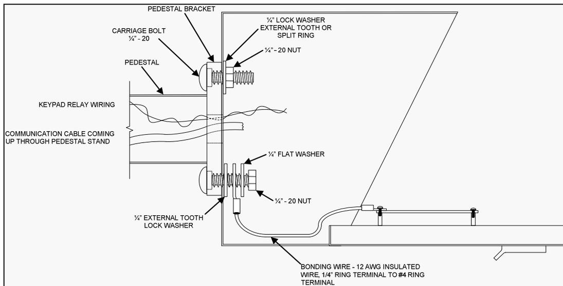
Figure 5 Enclosed Keypad (3200, 3200i, 1600, DaVinci) Surface Bonding Example
