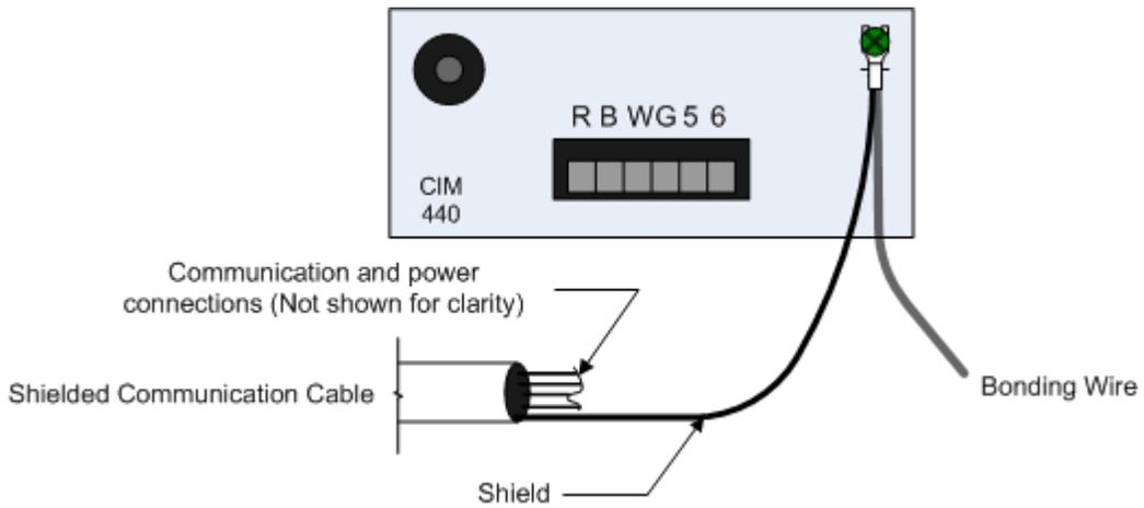
Figure 3 Bonding the Model 440 CIM.
