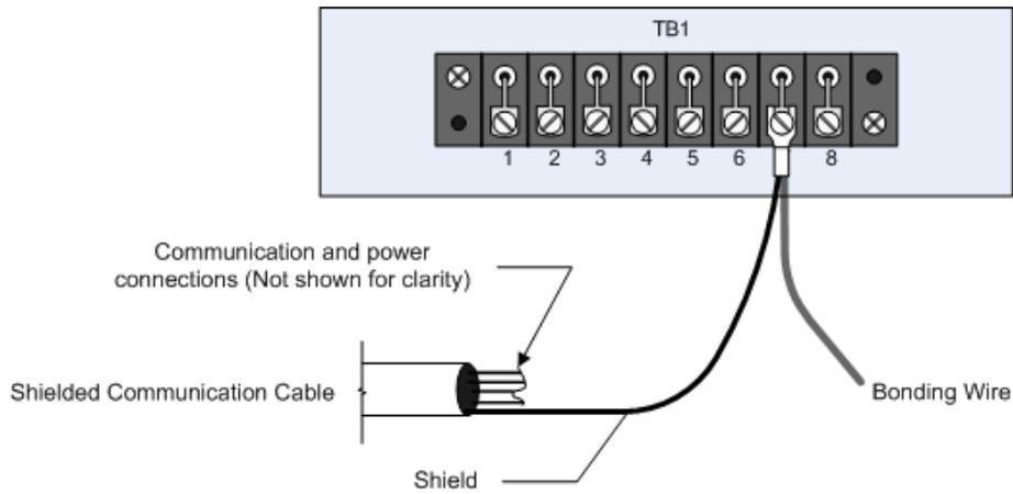
Figure 2 Bonding the Model 430 CIM.
