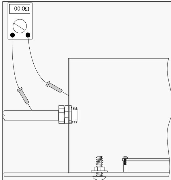
Figure 25 Continuity Testing – Conduit to Enclosure
