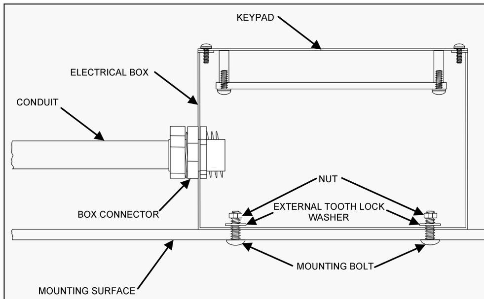
Figure 7 Keypad 314 Rubber/Metal Surface Bonding Example
