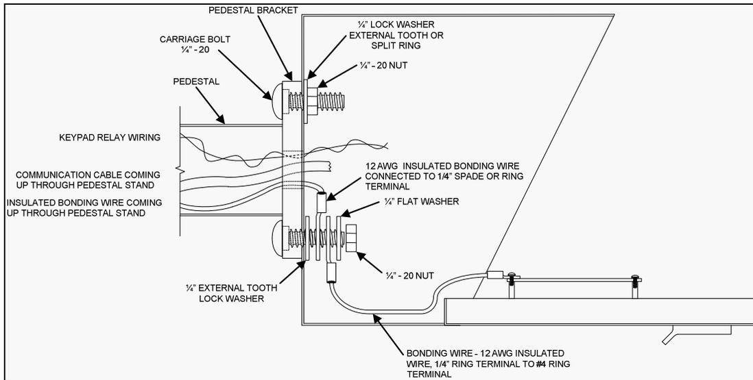
Figure 6 Enclosed Keypad (3200, 3200i, 1600, DaVinci) Wire Bonding Example
