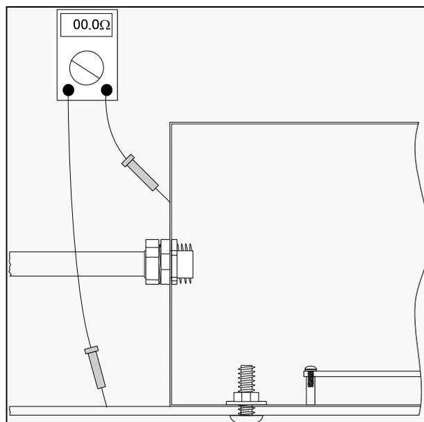
Figure 26 Continuity Testing – Mounting Surface to Enclosure
