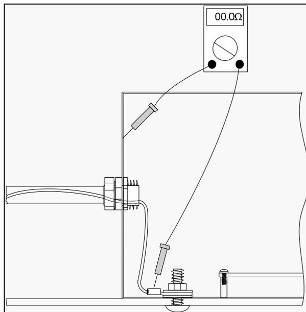
Figure 24 Continuity Testing – Bonding Wire to Enclosure
